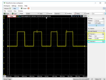
Figure 3 - Real-World Results for Voltage Drop Across Push Button
